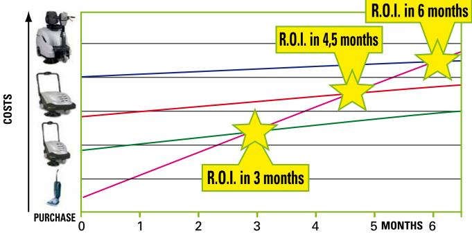
Note: calculation based on the average machine price, labour cost and surface of 300 sqm that has to be cleaned 5 day a week.
