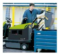
Effective discharge system thanks to separate controls for hopper raise and tilting
